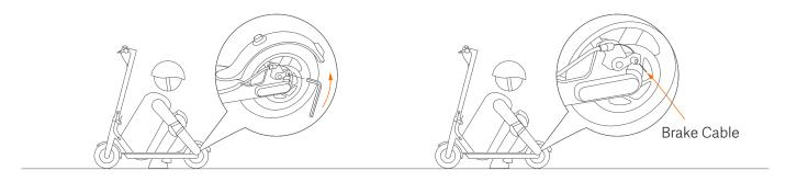
If the brake is too tight, use the 4 mm Allen key to loosen the screw on the caliper. Then slightly adjust the brake line (decrease the exposed length), and tighten the screw again. If the brake is too loose, loosen the screw on the caliper. Then slightly adjust the brake line (increase the exposed length), and tighten the screw again.
