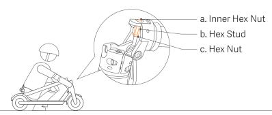
Long-term use of the scooter may result in loose screws, causing the handlebar stem to get unstable. If you notice the handlebar stem gets shaky when riding, follow the steps below.
