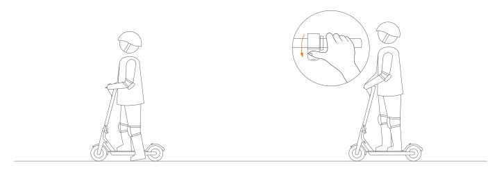
Step on the deck with one foot, and slowly kicks off the other on the ground. When the scooter starts to coast, put both feet on the deck and press the accelerator. Note: The accelerator initiates once the coasting speed exceeds 5 km/h.
