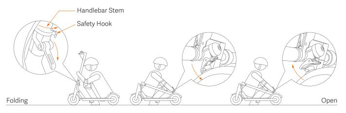
The scooter needs to be turned off before folding. Hold the handlebar stem, turn it counterclockwise to open the safety hook and open the quick release lever. Align the bell and the buckle and hook them. When opening, disengage the bell lever from the buckle on the mudguard. Fold the handlebar stem up, close the quick release lever and turn the handlebar stem clockwise to close the safety hook.
