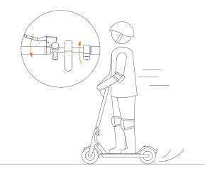
4. Release the accelerator and the kinetic energy recovery system (KERS) initiates automatically to brake slowly; squeeze the brake lever for a sudden brake. 3. When the scooter is at a full stop, the accelerator automatically turns off. To restart the scooter, it is necessary to repeat step 2.
