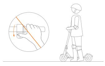
Do not press the accelerator when you're walking alongside the scooter.
