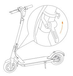
3. Tighten the screws onto both sides of the stem with the T-shaped Allen key.
