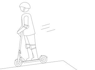
Do not accelerate when going downhill, and brake in time to slow down. When encountering a steep incline, you need to step off the scooter and push, do not risk riding up.
